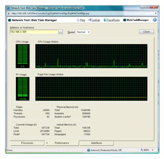
After you have identified a performance issue that is causing device performance issues, such as the Page File Usage indicating that the system memory is nearly at full capacity, you can correct the problem to bring the device performance back to normal.
