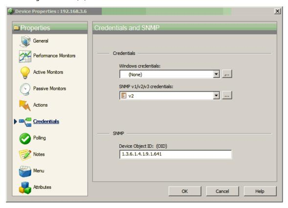
**Step 2: Configure a high capacity SNMP interface:**
