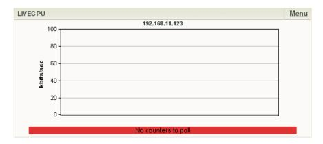
In the graphic above, the CPU Utilization Performance Monitor is not configured for the device. To correct this, you must go to the Device Properties for the device and configure the CPU Utilization Performance Monitor.
