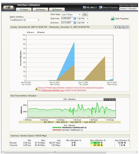
The graph now shows the total utilization of the interface as a percentage of the interface's total capacity. The numbers graphed are derived from the high capacity counters.
