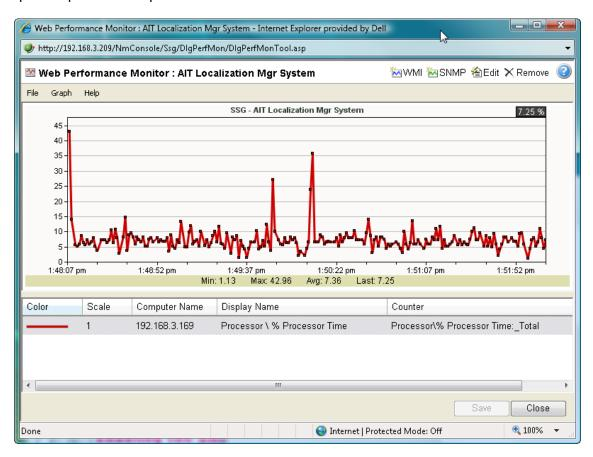
The graphs can be saved to the database and displayed on workspace views using the Split Second Graph - Performance Monitor workspace report or on the Web Performance Monitor tool. Multiple SNMP and WMI counters can be displayed on a single graph, and the color and scale of each graphed item can be individually configured.
