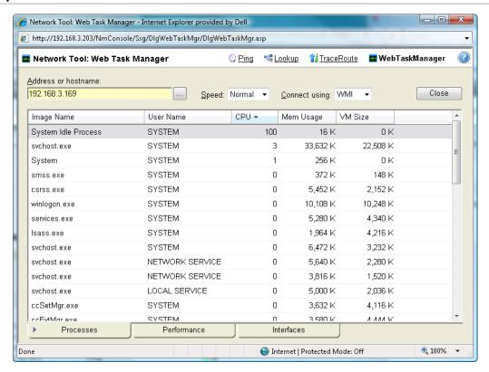
After you have identified a process that is causing device performance issues, such as an application executable like Outlook.exe running multiple instances of the program, you can correct the problem to bring the device performance back to normal.
