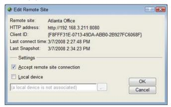
6 The **Accept remote site connection** option is selected by default. It allows users, with rights, the ability to select or deselect (from the Central Site) the option to accept connections from Remote Sites.
